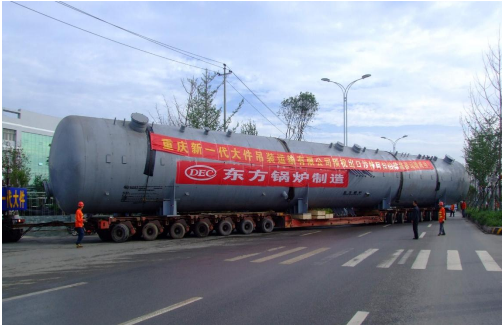
Headless deaerator for Saudi Arabia Rabigh 600MW power plant project
